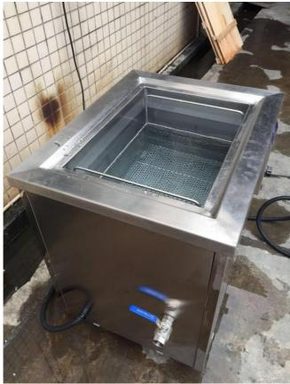
2 Put the clening items in, the cleaning items should fully immersed in the water. For oil removed, chemmicals is necessary.
